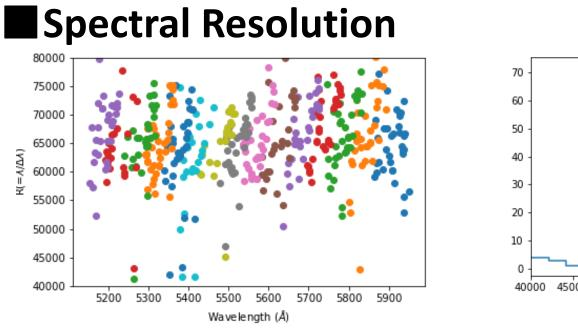
The spectral resolution is R~65000 based on the measurements with the spectrum of the ThAr light source.
