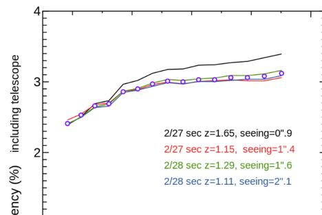
The efficiency of GAOES-RV with the telescope is 2.5-3% in the observation wavelength range. The actual observation efficiency depends on the atmospheric extinction and the efficiency of the
