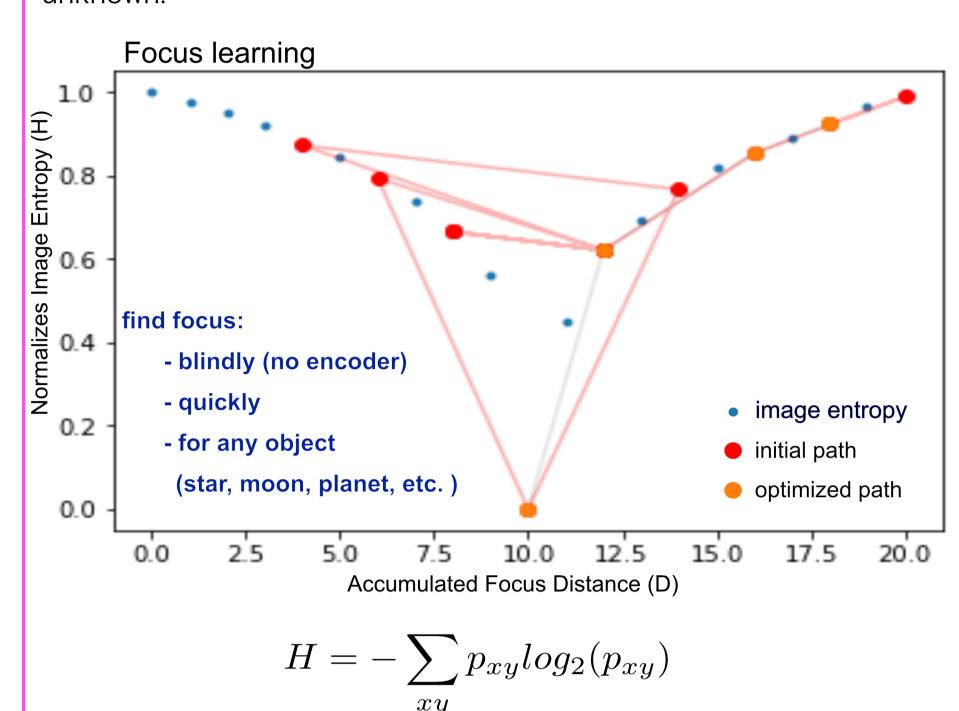
The focus between the The figure shows the estimated shortest path to lowest entropy focus from any position. dH/dD is used to anticipate the stepping distance for each point
